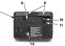
**To activate the thermometer,** open the battery compartment in the back of the unit (Fig. 2, Callout 12) by lifting the left side of the hinged door with your fingertip. Remove the battery activation tab. The beeper will sound quickly four times. Discard the tab and swing the battery compartment cover shut.
