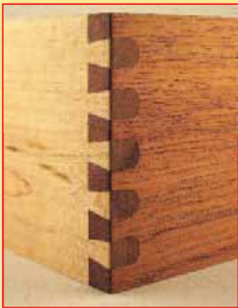
Cuts Through Joints
