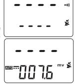
To match the receiving channel of your GT310 to the transmitting channel of the second multimeter, press and hold the Hold/CH button, and then press it briefly to cause the lower readout to show CH-0. Quickly (within 10 seconds), press the Select/0-9 button as many times as needed until the channel number on the lower readout matches the transmitting channel number of the second multimeter.
