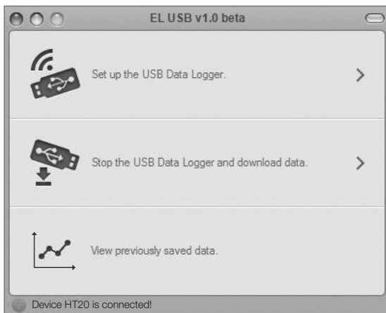
Fig. 2. The three options made available by plugging the HT20 into a USB port
