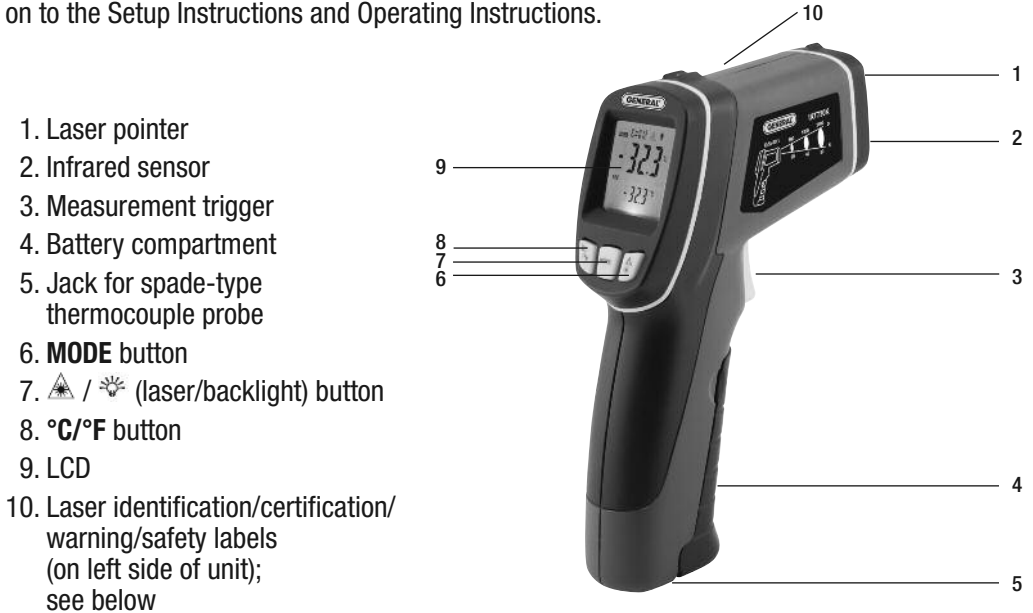
Fig. 1. All controls, indicators, connectors and other physical features of the IRT730K
