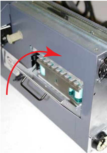
Analyzer Filter Door
