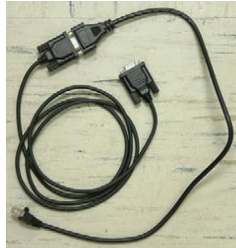
Figure F-5 -- Debugging Cable
