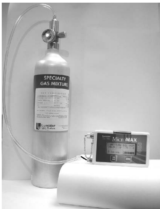
Figure 6 Calibrating the MicroMax Pro
