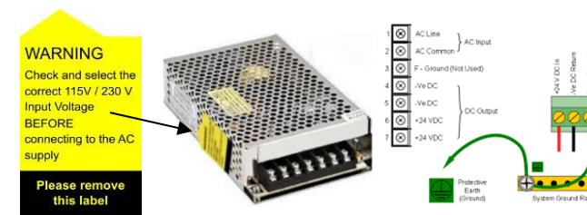
Figure 4. Switched Mode Power Supply (SMPS) Connections
