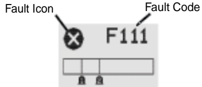
Figure 12. General Status Fault detail
