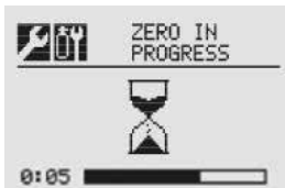
Figure 195. Zero Calibration in Progress
