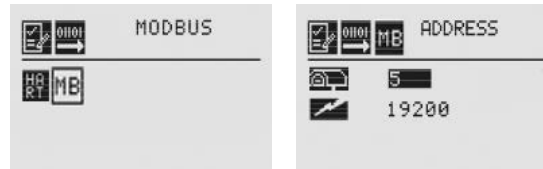
Figure 182. Modbus Configuration Display screen
