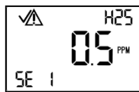
One sensor Installed
