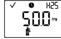
Bump test apply gas
