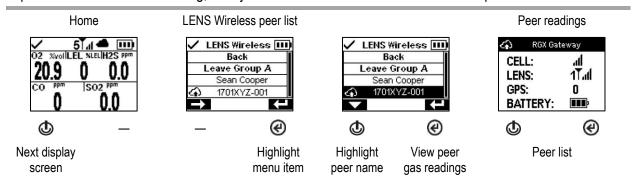
Figure 5.9 Access peer gas readings
