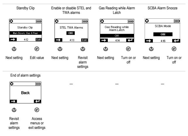
Figure 4.2.D Navigating and editing alarm settings
