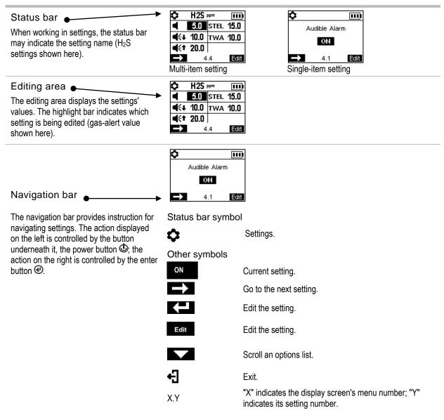
Figure 3.2.D Reading the display while working in settings
