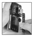
Unscrew, lift, and remove the battery from the diffusion instrument; store it for future use.
