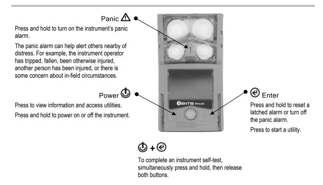
Figure 5.1 Using the buttons during operation
