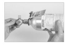
Holding the regulator, turn the calibration gas cylinder in a clockwise direction to tighten.
