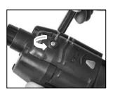
Loosen the pump door screw.
