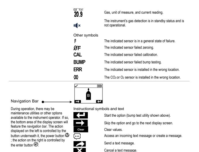
Figure 3.2.A Reading the display during operation
