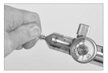
Connect either end of the calibration tubing to the regulator's nipple.
