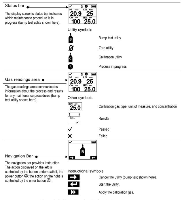
Figure 3.2.C Reading the display during maintenance
