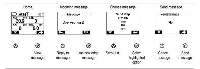
To initiate messaging, repeatedly press the power button (③) to reach the *cellular battery* screen. The message symbol (⑤) will display in the navigation bar. Press the button below the symbol to display the "choose message" list. Scroll through the list, then highlight and send the desired message.
