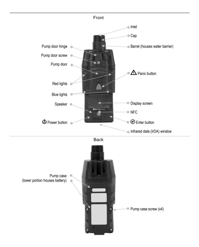
Figure 3.1.B Hardware overview aspirated instrument
