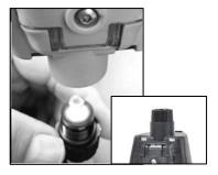
Invert the instrument. Place the new internal filter in the inlet barrel of the instrument.
