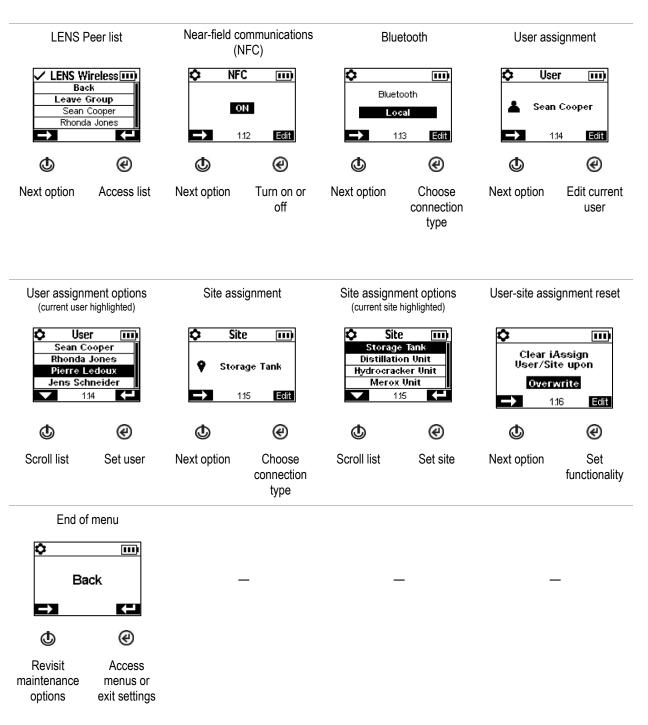
Figure 4.2.A Navigating and using maintenance options
