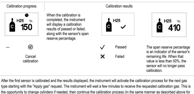
H<sub>2</sub>S) until all calibration gases have been applied.
