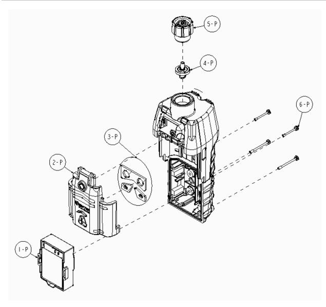
Figure 8.2 Pump module diagram
