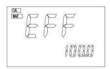
This screen will display the efficiency of the pH electrode from its last calibration. This screen is for user information only and will automatically change to the 4mA setting after 4 seconds.
