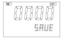
This screen selects the password number for this unit. The user can use [♠], [♥] or [▶] keys to input the new password. Pressing the [OK] key will save the password number and LOCKS the unit. You will not be able change any setting or turn-on
