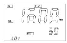
This screen is essentially the same for the four relays. Take note of the blinking character as there are 3 values to input for each relay. The user has to input the SET-POINT first then the HYSTERISIS and finally the RELAY ACTION.
