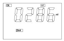
This screen will let the user change the 20 mA value. The user can use [♠], [♥], [▶] or [OK] keys to input new 20mA value. This value is used for scaling the 4-20mA ANALOG OUTPUT. (For detailed explanation see chapter VI. 4-20 mA OUTPUT.)
