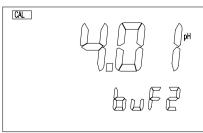
This screen selects the buffer for slope calibration. The user can select "1.68pH", "4.00pH", "4.01pH", "9.18pH", "10.01pH" or "12.46pH". Press the [♠] or [▼] keys to select the buffer then the [OK] key to save your selection.
