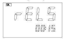
This screen set the ON TIME delay in MINUTES:SECONDS for the RELAY 5. The user can use [♠], [▶] or [OK] keys to input the new ON time. You can only turn-ON the WASH relay if the unit is UNLOCKED.
