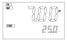
This is the actual pH calibration. The initial display will be the chosen buffer for pH BUFFER I SELECT. The "STAND" annunciator will blink indicating the unit is waiting for the user to start the calibration. Put the cleaned electrode and
