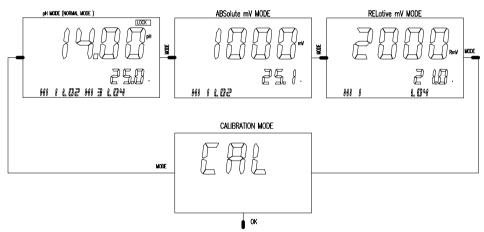
Turning ON the unit will always display **MAIN** display mode. This instrument is designed to provide 4 distinct measurements:
