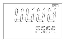
You will only see this screen if the unit is LOCKED. To change any settings or calibration you need to unlock the system to remove the "LOCK" message. You can use [♠], [▶] or [OK] keys to enter the correct 4-digit number on the
