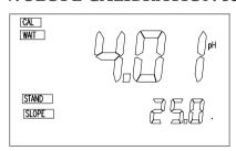
After finishing the Buffer I calibration the unit will move to this screen. The initial display will be the chosen buffer for **pH BUFFER II SELECT.** The "**SLOPE**" annunciator will blink indicating that the unit is waiting for the user to continue the calibration.
