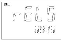
This screen selects the ON TIME delay in **MINUTES:SECONDS** for the **RELAY 5.** The user can use [♠], [♥], [▶] or [OK] keys to input the
