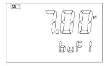
This screen selects the buffer for standardization calibration. The user can select "7.00pH" or "6.86pH". Press [▲] or [▼] keys to select the buffer then the [OK] key to save your selection.
