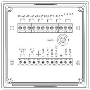
Before connecting the probes, relays, analog output, RS485 and power cord be sure that you are inserting to the right terminal as shown above. Remember that the unit is ON once the user plugs in the power cord to an AC power supply.
