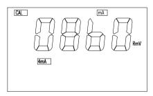
This screen will let the user change the 4 mA value. This value is used for scaling the 4-20mA ANALOG OUTPUT.
