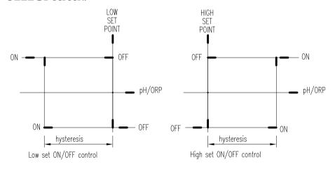
The figure above shows how the relays react to user set point, hysteresis and reading.
