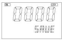
This screen selects the password number for this unit. The user can use [♠], [♥] or [▶] keys to input the new password. Pressing the [OK] key will save the password number and LOCKS the unit. You will not be able change any setting or turn-on
