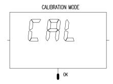
Pressing the [OK] key at the CAL mode will bring-up the PASSWORD CHECK display if the unit is LOCKED. If the unit is not locked, the unit will skip the PASSWORD CHECK screen and go directly to CALIBRATION SELECT screen.
