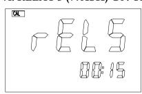
This screen selects the ON TIME delay in MINUTES:SECONDS for the RELAY 5. The user can use [▲], [▼], [▶]or [OK] keys to input the new ON time. You can only turn-ON the WASH relay if the unit is UNLOCKED.
