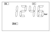
This screen will let the user change the 20 mA value. this value is used for scaling the 4-20mA ANALOG OUTPUT.
