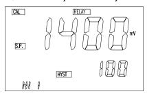
This screen is essentially the same for the four relays. Take note of the blinking character as there are 3 values to input for each relay. The user can use [♠], [♥], [▶]or [OK] keys to input the SET-POINT first then the HYSTERISIS and finally
