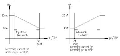
The above figure shows the relationship between Reading,  $U_{4mA}$  &  $U_{20mA}$ .
