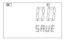
This screen selects the unique ID/address for the unit. Your RS485 communication program must also use this same ID/ address to communicate with this unit. The user can use [♠], [♥], [▶]or [OK] keys to input the new ID/address.
