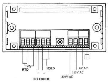
WIRING DIAGRAM FOR RTD MODEL DRAWING 5
