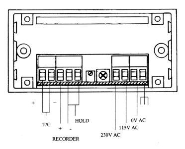
WIRING DIAGRAM FOR T/C MODEL DRAWING 4
