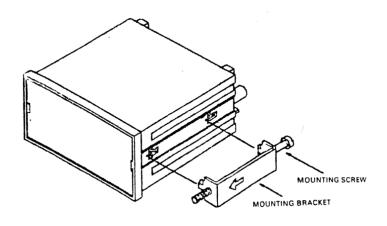
PANEL METER WITR MOUNTING BRACKET AND SCREW DRAWING 2
