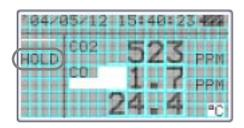
"HOLD" indicator appears on the display to indicate that the reading shown is held.
