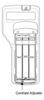
In case you find the LCD display of Main Body too dark or too light, there is an adjusting volume at the back, bottom of Main Body, inside the battery cover.
