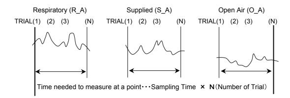
Respiratory Air:  $R_A = \Sigma TRIAL(N)/N$ Supplied Air:  $S_A = \Sigma TRIAL(N)/N$ Open Air:  $O_A = \Sigma TRIAL(N)/N$ \*\* Ventilation Ratio (%OA)
