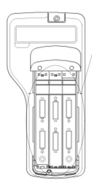
④Insert the battery observing the polarity. This instrument requires 6 AA size batteries. Use only AA size Manganese (R6), alkaline (LR6) or Ni-Cd batteries for replacement.
