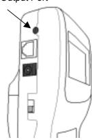
Of the output range, the low end will be set at 0V and the high end will be set at 1V. Data output interval is always 1 second.
