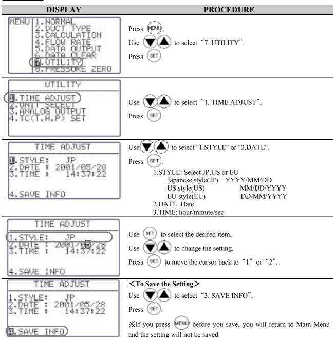
X Date of the output to the display or printer depends on this setting. But the style of the output to digital port (RS-232C) is fixed as Japanese style.
