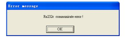
Confirm the communications cable is properly attached and the baud rate settings are correct.
