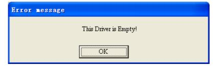
3) If there is a communication failure between the computer and the instrument, the following message will be displayed:
