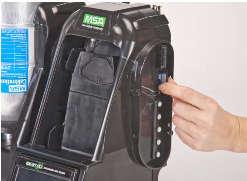
Fig. 13 SD or SDHC Memory Card Installation
