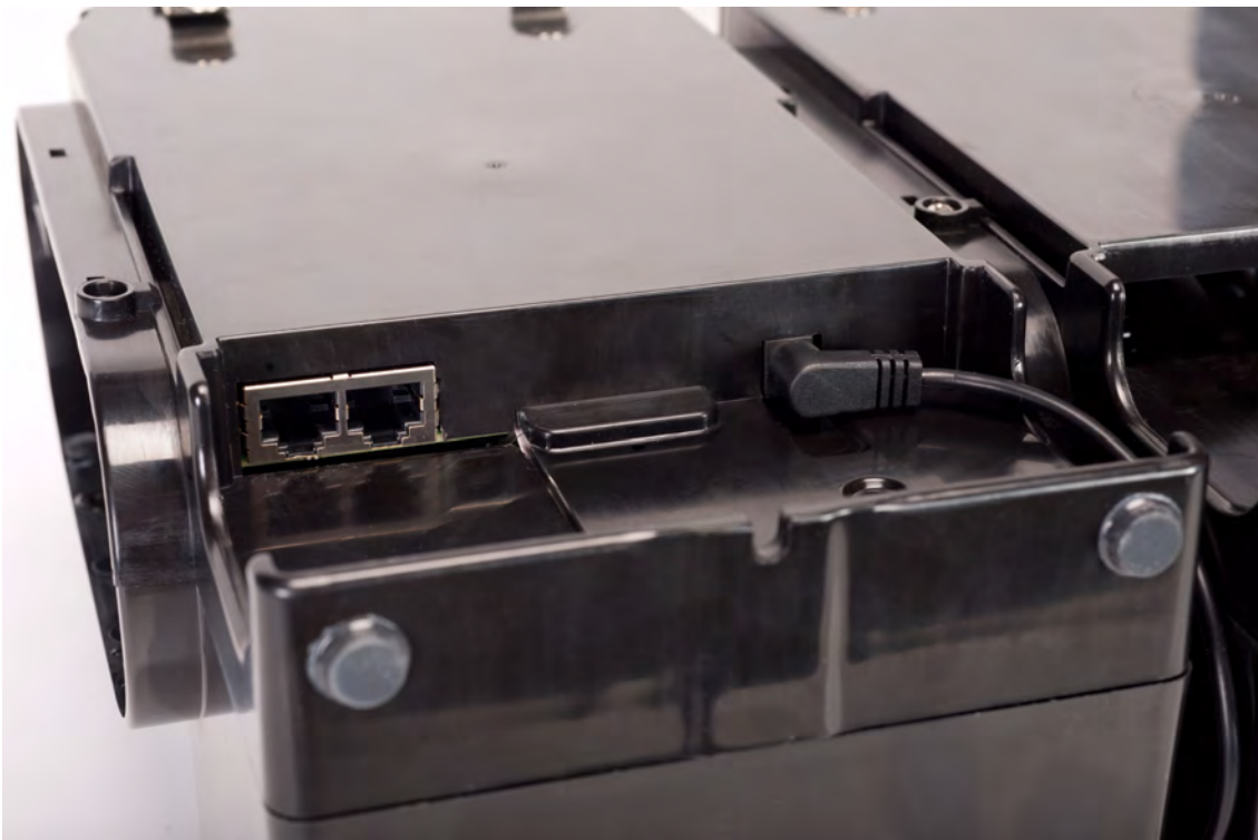
Fig. 6 Test Stand Ethernet jacks
