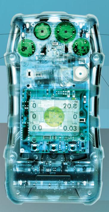
MSA XCell SO<sub>2</sub>, Cl<sub>2</sub>, or NH<sub>3</sub> Sensor
