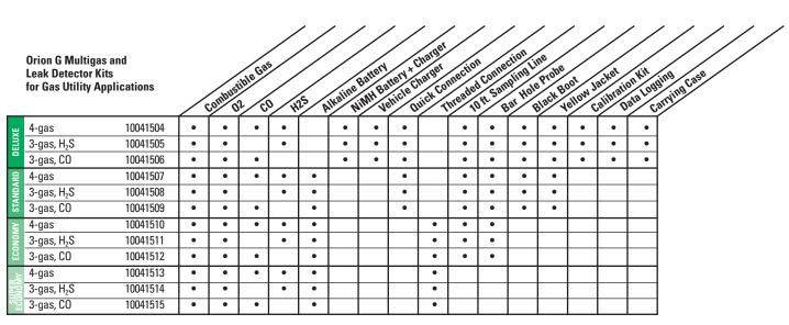
For customized assemble-to-order Orion G Multigas and Leak Detector configurations or replacement parts, please request ATO bulletin #0816-45-MC.
