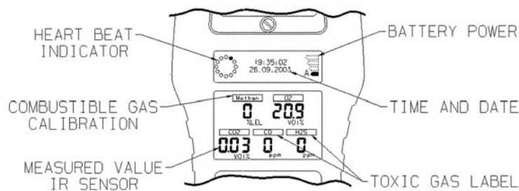
Figure 3-3. Heartbeat, Time & Date, and Battery Life Indicator
