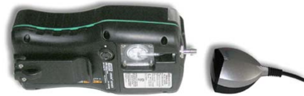
Figure 5-5. Attaching the Infrared Adaptor to the Instrument
