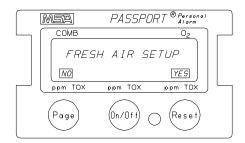
Figure 2-25. Fresh Air Set-up
