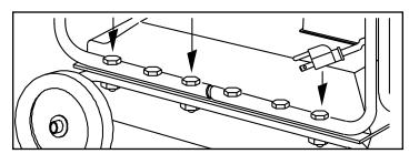
3. Attach safety guard to front of heater with screws provided.
