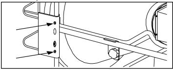
4. Attach Radiant Visors to the top and bottom rear of the Radiant Cone Assembly using extra screws included.
