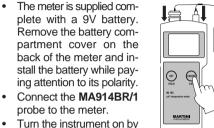
• Connect the MA914BR/1 probe to the meter. Turn the instrument on by pressing the ON/OFF key. At start-up, the LCD
