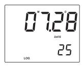
The instrument then displays the amount of free log space for about one second and returns to normal measurement mode (e.g. 45 records free).
