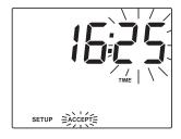
Press the arrow keys to change the blinking value.
