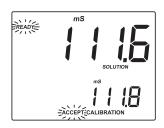
Press the GLP/ACCEPT key to confirm calibration.
