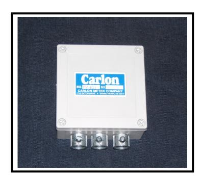
The Carlon Meter Power Pack 101 provides a means to have separate, independent circuits signaled from the output pulse signal of a dry contact meter (Carlon JSJ Series, for example) or a reed switch or "hall effect" meter. Sometimes called a "splitter", the unit provides two isolated output signals, which carry independent voltage from two respective sources. Sources can be a controller, a remote counter, or some other receiving device.
