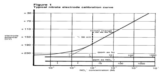
millivolt mode. The measured electrode potential in mV (linear axis) is plotted against the standard concentration (log axis). In the linear region of the curve, only three standards are necessary to determine a calibration curve. In the non-linear region, additional points must be measured. The direct measurement procedures given are for the linear portion of the curve. The non-linear portion
