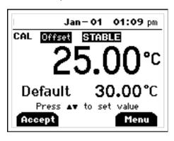
Use the ▲ or ▼ keys to adjust the value to match known temperature standard. Press *F1* to accept.
