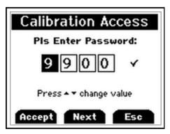
Before go into the calibration mode, must enter the password. Press F2 to change to the next digit. (Default Password is 9900) There are two calibration options:
