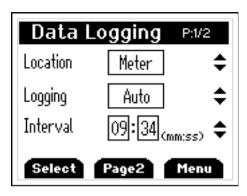
Press recall ▲ or log ▼to choose logging methods as auto or manual. If it is auto logging, using recall ▲ or log ▼to set time interval. Its range is from 0min to 60min
