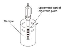
After immersing the electrode in the sample, lightly stir the electrode around to optimize the contact area with the sample and remove any air bubbles.
