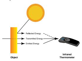
Infrared thermometers sense emitted, reflected, and transmitted energy from an object and translate this information into a temperature reading. In essence, energy passes through the unit's optical system and is converted to an electrical signal at the detector. The signal is then displayed or converted to a standard output (°F or °C).
