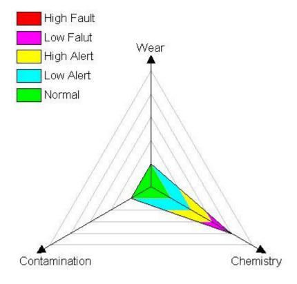
A plot may show high wear but otherwise healthy oil, good oil contaminated with water, or any other combination of problem. It is not unusual for an oil to first experience a Chemistry problem as additives are depleted and soluble contaminants build up. Left uncorrected, the oil problem can develop a Contamination problem, and eventually an abnormal Wear condition.
