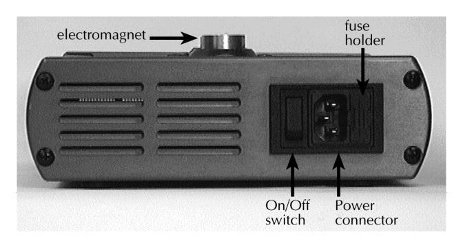
After connecting the interface cable, plug the 110/220 volt power cable into the OilView® Quick-Check Analyzer unit and into a 110/220 volt outlet, and then turn the unit on. The analyzer should give a three-tone output and display the OilView® Quick-Check copyright message on its LCD screen.
