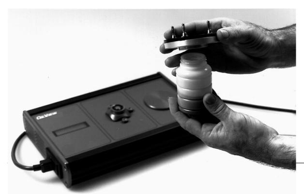
Vigorously shake the sample bottle after making sure that the cap is screwed on tightly. This must be done to ensure that the contaminants are evenly dispersed in the sample. The bottle should be shaken 15 seconds or until no sediment can be seen on the bottom of the bottle after it has been inverted. In extreme cases, it may be necessary to stir the sediment from the bottom of the bottle using a clean plastic or glass rod before shaking.
