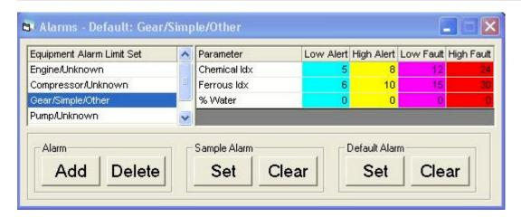
Test results are displayed with colors that correspond to the calculated alarm level. This facilitates a quick assessment of the sample status.
