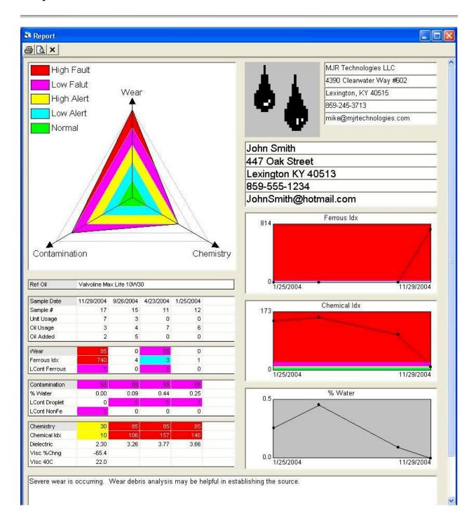
The Report window summarizes test and trend data for a sample. A non-blank "Equip. ID" is required before data can be displayed. Prior samples with a matching "Equip. ID" will be retrieved for historical trending. "Sample #", "Unit Usage", "Oil Usage", "Oil Added", "Visc 40C", and "Comments" for the current sample may be modified by
