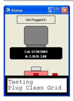
The Status window will reflect the various states and conditions of the OilView® Quick-Check analyzer. The text status may be easier to read then the device display. Also, the Calibration information can easily be verified for correct date and dielectrics. This window is not required for successful operation of the system and may be closed, minimized, or moved if desired.
