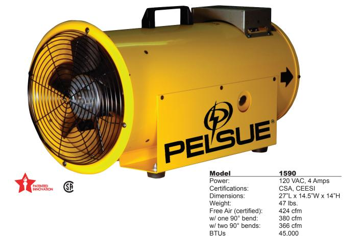
**Model 1590**, one-piece, Axial Propane Heater/Blower, provides fresh warm air. It is extremely efficient requiring only 45,000 BTU's of input to get a 125° heat rise. Certified for ventilating confined spaces with or without heated fresh air via air ducts. This model is available in both North American and European voltages.
