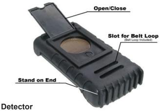
Internal Halogen-quenched, uncompensated GM tube with thin mica window, 1.4-2.0 mg/cm2 areal density. Effective diameter of window is 45 mm (1.77 in.). Radiation symbol on front label marks the center of the detector.
