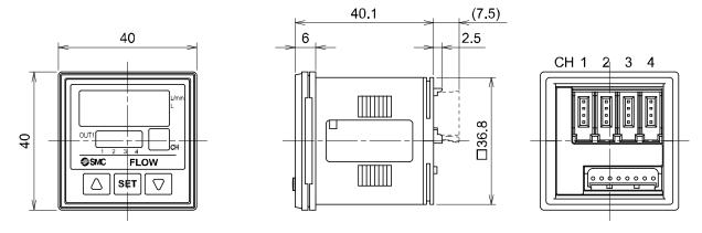
PF2□20□ + panel mount adapter (ZS-26-B) + front protective cover (ZS-26-01)
