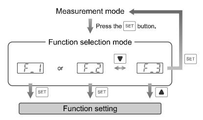
\*: When the output mode is set to instantaneous output mode, [F\_1] is displayed. When the output mode is set to accumulated output mode, [F\_2] is displayed. When the output mode is set to accumulated pulse output mode, [F\_3] is displayed.
