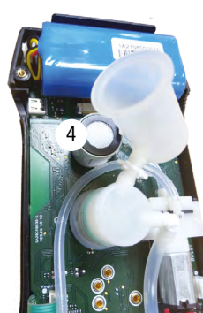
New sensor connected to electronic board
