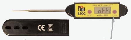
3. Press and hold the D-H/CAL button for approximately 8 seconds until "CAL" is displayed. "CAL" will display for approximately 2 seconds and then the C series thermometer will return to normal operation. Calibration is complete.
