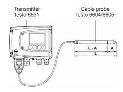
L = Probe length L-A = Probe length – length protective cal A = 35 mm
