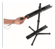
2 If necessary, feed the probe cable through the cable holder (1).
