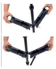
9 Secure the probe mount by closing the snap lock.
