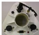
Figure 3: The power switch and Scan/Receive light is located on the bottom of the WeatherHawk
