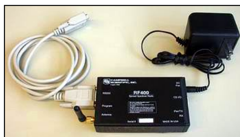
Figure 11: Radio connections. The serial cable (left) connects to the port labeled RS232 and the AC adapter connects to the port labeled DC Pwr input.
