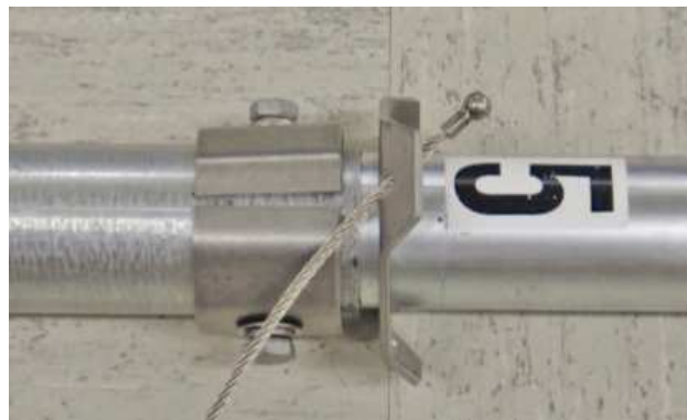
Figure 24: Mast Section 5 and Guy Ring/Collar Assembly
