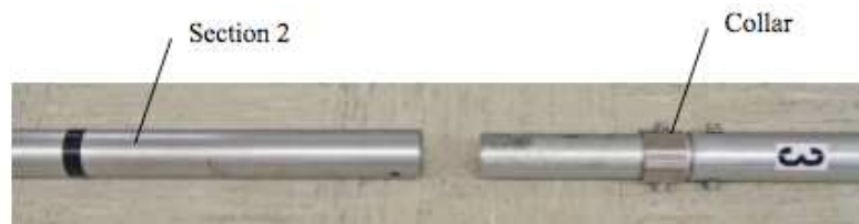
Figure 15: Mast Section 2 and Mast Section 3
