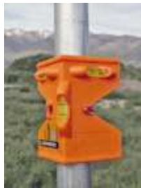
Figure 35: Pole Level Ensures Vertical Mast.
