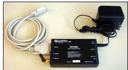
Figure 6: Radio connections. The serial cable (left) connects to the port labeled RS232 and the AC adapter connects to the port labeled DC Pwr input.
