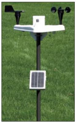
WeatherHawk provides real-time weather measurements and calculates  $ET_0$  on an hourly and daily basis.
