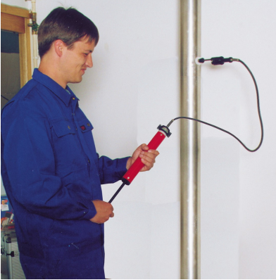
Fig. 4: Extracting the smoke gas
