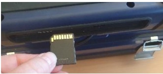
Fig. 9: Insert SD card correctly
