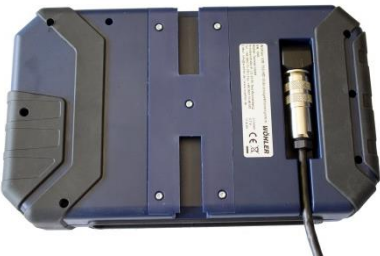
Fig. 11: Camera cable fed through guide
