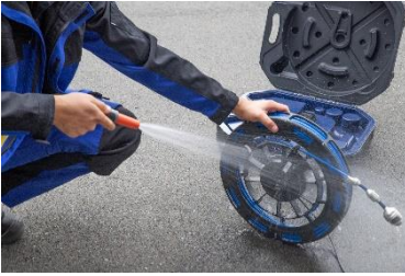
Fig. 57: Cleaning the viper and the rod
