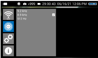
Fig. 32: Locator detection with 8.9 kHz transmission frequency selected
