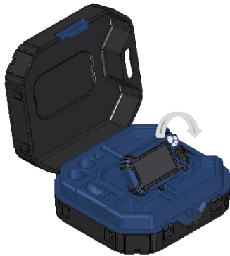
Fig. 10: Tilt the monitor up and down
