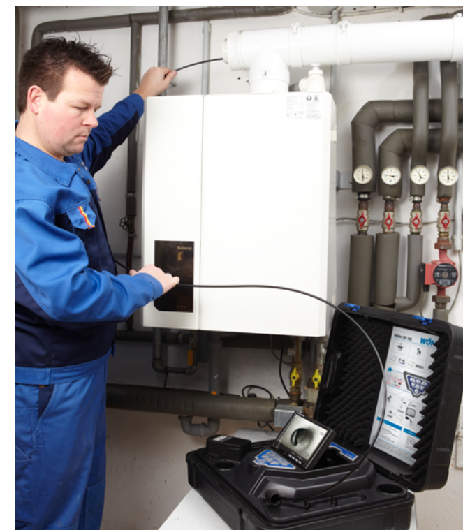
The Wohler VIS 200 series camera is a valuable tool in a wide range of applications including the analysis of flue gas installations.
