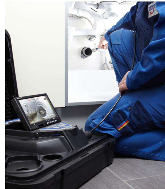
The robust color camera head is waterproof to IP 68 rating. With a diameter of just 1" it easily negotiates bends in pipes of 1.5" and larger.
