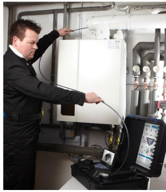
The 360° pan- and 180° tiltable color camera head easily negotiates 90°
