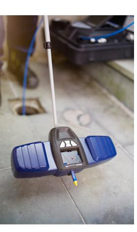
Contractors and their customers are able to save considerable time and money by utilizing video inspections to visualize leaks and document damaged or soiled sections of pipework. The Wohler L 200 Locator also locates the radio signals transmitted by the camera head of the precisely in a clear-cut graphic on the how the Wohler L 200 makes locating simple: The Locator can be attached to
