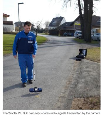
head through concrete and asphalt to save time and money in repairs.
