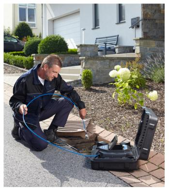
The robust color camera head is waterproof to IP 67 rating. With a diameter of just 1.5" it easily negotiates bends in pipes of 2.5" and larger.
