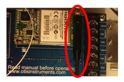
6. Run the u.fl cable from the Laird radio to one of the u.fl connectors next to one of RPSMA connections.
