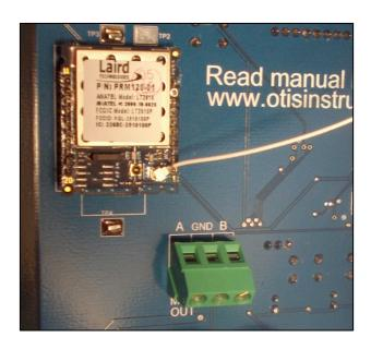
3. Secure the Laird radio to the terminal board using the provided zip ties.
