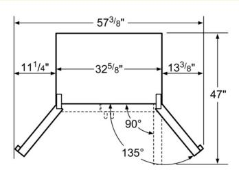
Drawers can be pulled out with door open 90°. Drawers can be taken out with door completely open.
