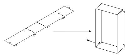
STEP 4: Attach the ventilation ducts as shown below.
