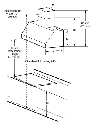
**Note:** Typical overhead cabinets are 12" deep. For cabinets of greater depth, place spacer of non-combustible material behind hood.
