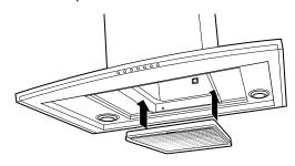
Install the black charcoal filter into the center opening.
