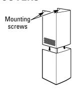
The inside duct piece must slip into the folded ends of the outer section.
