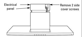
Remove one screw on each side of the cover on the electrical panel. Lift off the cover and set aside with screws.
