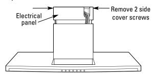
Remove one screw on each side of the cover on the electrical panel. Lift off the cover and set aside with screws.
